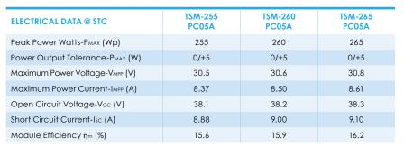
STC: Irradiance 1000 W/m², Cell Temperature 25°C, Air Mass AM1.5 according to EN 60904-3. Average efficiency reduction of 4.5% at 200 W/m² according to EN 60904-1.
