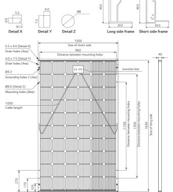
The distance between the center of the mounting/grounding holes
