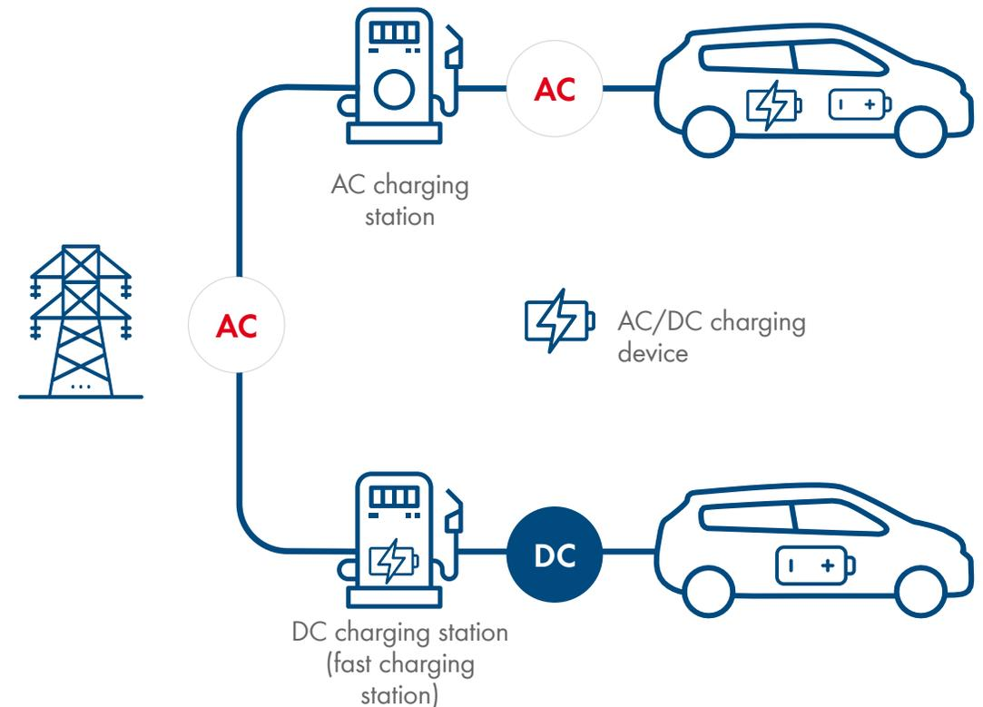
> **An AC charging station (wallbox) is NOT an inverter (AC in/AC out)**
