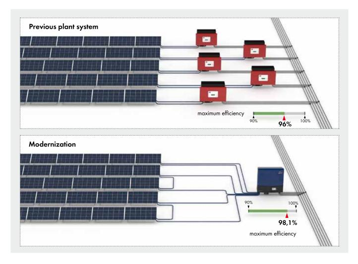
Another plus: With the SMA Upgrade, the PV system automatically complies with the VDE application guide 4105 according to the 2012 Renewable Energy Sources Act (EEG). Furthermore, the integration of the latest SMA communication products, which you can offer to your customers, is also possible.
